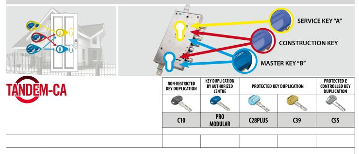
TANDEM-CA with common construction key is a master key system consisting of a pair of MOTTURA CHAMPIONS® to be installed on a double cylinder lock. Cylinder "A" has a service function; cylinder "B" has a master key function. The construction key can open both cylinders and will be disabled by the 2 service keys "A" and by 5 master key "B". The CHAMPIONS® master key (B) can open the service CHAMPIONS® (A), but not vice versa.
