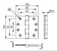
Included in a successful fire test to BS EN1634 Part-1. Suitable for use on 60 minute timber fire doors (Intumescent pack must be used)
