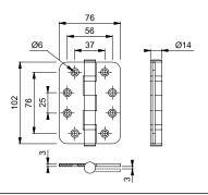
Included in a successful fire test to BS EN1634 Part-1. Suitable for use on 30, 60, 90 and 120 minute timber (Intumescent pack must be used) and 240 minute steel fire doors
