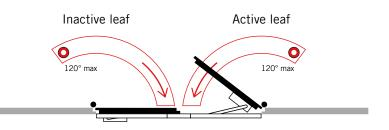
Adjustable strength. Hydraulic speed control. Back Check. Delayed action
